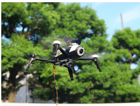
Figure 1: Flying tethered drone with prolonged flight time
