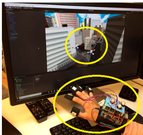
Figure 5: Swarm of drones controlled in virtual reality with the help of the tactile glove.
