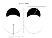
Figure 1: The expressive eyes are defined by varying two parameters of overlapping circles. This way the autonomous expression is easily achievable.
